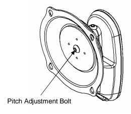
Figure 15. Adjust Pitch Tension
